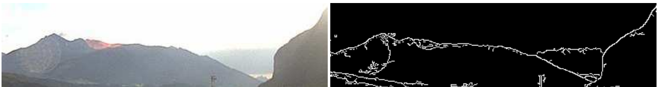
Figure 3: original image (left), Canny edge detector (right)
