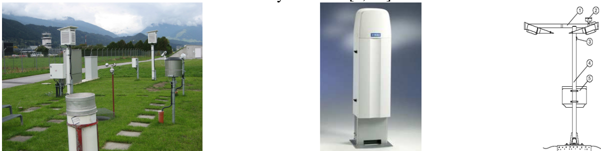
Figure 1: Classic airport sensor system: meteorological instrumentation and equipments (left), ceilometer (middle), sketch of a visibility sensor (right).
